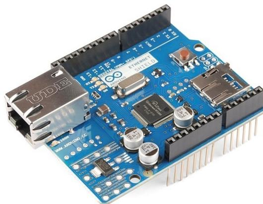
Figura 8 – Arduino Ethernet Shield
