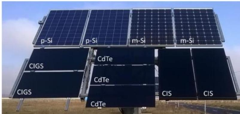
Fonte: Analysis of the Conversion Efficiency of Five Types of Photovoltaic Modules During High Relative Humidity Time Periods, Burduhos et al. [2018]
