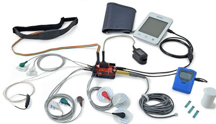
Figura 5 - *E-health sensor platform* completo. Fonte: COOKING HACKS, 2014.
